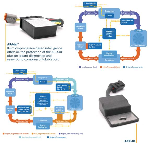
Detects rapid cycling and protects from under-voltage. The ACX-10 eliminates heat build up as well as delays the A/C clutch engagement to extend the compressor's life.
