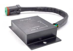
The Inclinometer measures the acceleration forces on the vehicle in 3 axes (x,y,z) as well as the rate of change of the angular position of the vehicle in 3 axes using a built in MEMS sensor.
